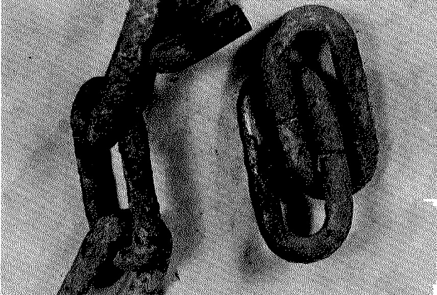
Photo #12 & #13. Half-inch special chain, non-galvanized, showing the results of corrosion.
