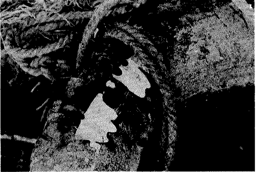
Photo #9. Tire casing chafe due to fiber rope abrasion.
