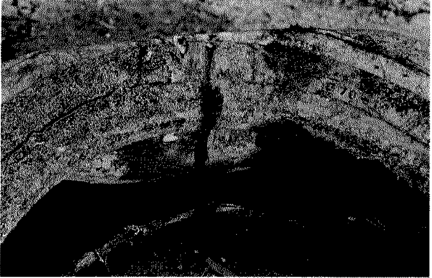
Photo #6. Tire casing depicting a typical cut due to wire chafe.
