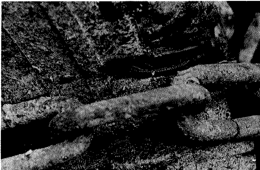
Photo #14. Cut into tire casing as a result of half-inch special chain abrasion.
