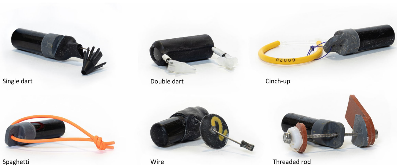
FIGURE 1 Six methods for attaching acoustic transmitters to fish
