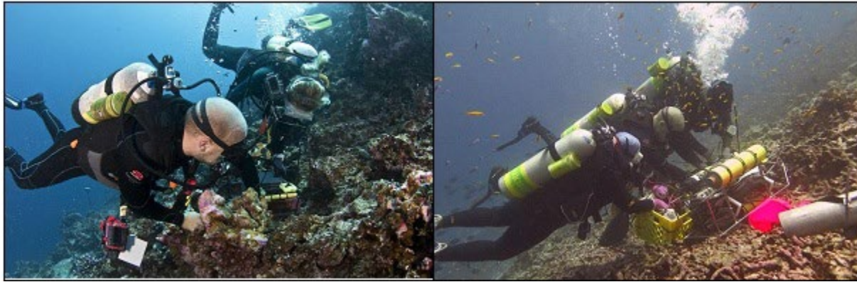
Figure 5. Examples of divers deploying instruments such as water sampling units and the conductivity, temperature, depth, and pH sensors (Photo source: NMFS Pacific Island Fisheries Science Center)
