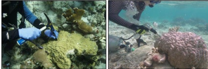
Figure 12. Examples of collecting small coral cores (Photo source: NOAA [left]; Johnston Applied Marine Science [right])
