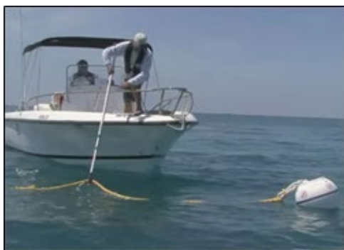
Figure 41. A boater secures the buoy mooring line to anchor his vessel (Photo source: NOAA)
