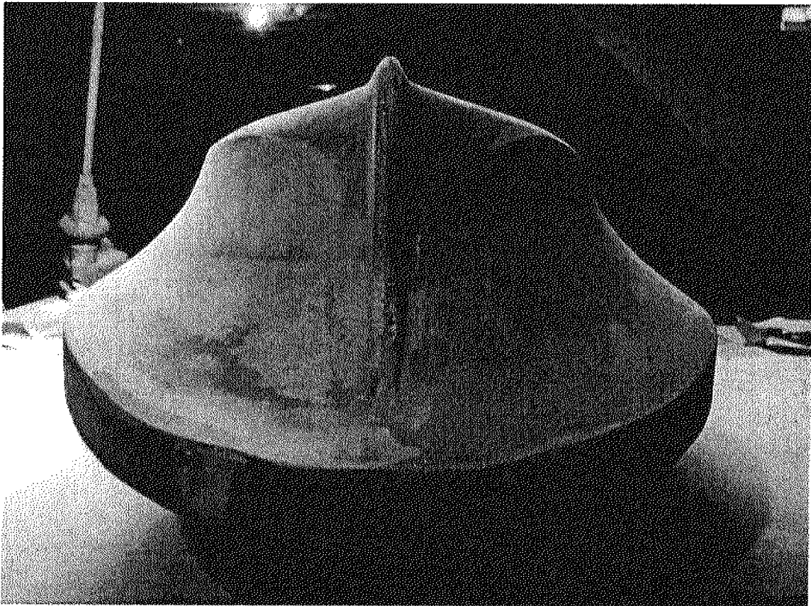
Figure 24 - Bow after Repair and Final Hand Sculpting
