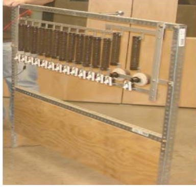
Figure 35: Load Controller, using 3.1 Ohm, 300 Watt Power Resistors
