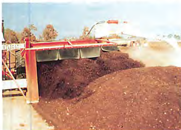
Figure 4.3 Method used to place crab scrap and scallop viscera into opened windrows.
