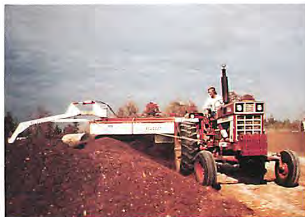
Figure 4.4 WILDCAT™ machine turning crab scrap compost (front view).
