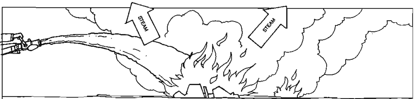
Figure 4-18. Water cools a fire and removes the oxygen as it flashes to steam.
