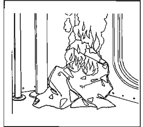
Figure 4-2. Oil-soaked rags in a warm, unventilated corner are all it takes to cause a fire.
