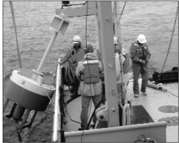
A buoy deployed to tether CTD/DO profilers is recovered from the Stratford Shoal area of Long Island Sound by the crew of the R/V Connecticut .
