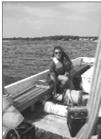
UConn Marine Sciences Ph.D. candidate Jamie Vaudrey deploys YSI continuous monitoring sondes in Mumford Cove. These instruments profile the water column every hour for a two-week deployment, providing information on water column characteristics.
