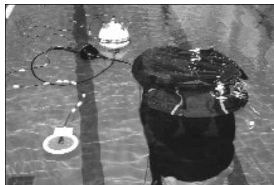
The in-situ multi-sensor float instrument used to measure heat flux.
