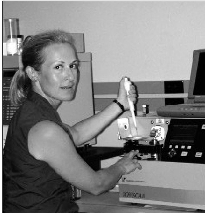
Researcher Claudia Koerting, above, has found that the Ionscan ® (right), an ion mobility spectrophotometer routinely used by airport security systems and the military for detecting explosives and narcotics, can be applied to the rapid detection of bacteria in food, and presence of organisms that might cause harmful algal blooms. This technology is faster and less expensive than traditional methods.
