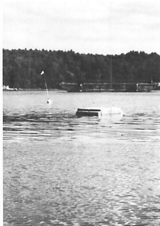
Flounder cage in position down stream from the nuclear power plant, Wiscasset, Maine. Flagged buoy beyond cage marks continuous water temperature recorder.
