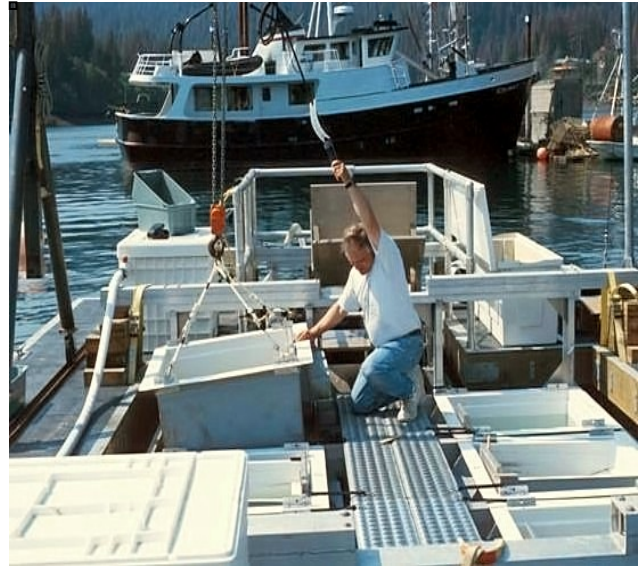
Original 1995 FLUPSY at Halibut Cove, Kachemak Bay. With an efficient paddlewheel pump, water flows through bins of oyster seed providing abundant food. Seed can grow from 5mm to over 25mm in length with three months of growout (Photo by I. RaLonde)
