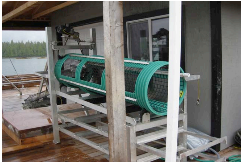
A tumbler/sorter at Mike Sheets' farm south of Naukati. This unit was manufactured in a Ketchikan welding shop.
