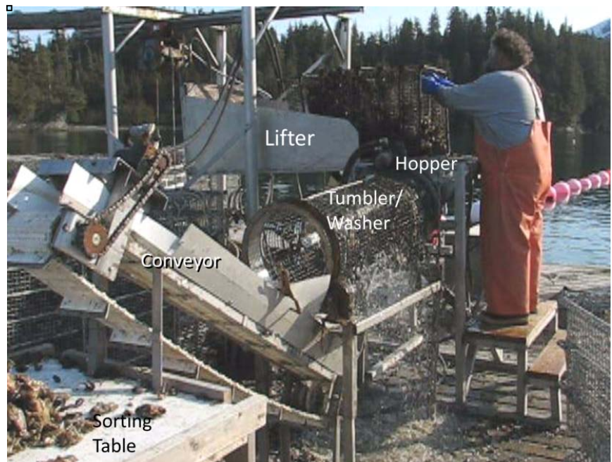
Lifting system at Aguiar's farm that shows the operation from lifter to cleaning and sorting. The entire process is mechanized and requires no bending or heavy lifting.
