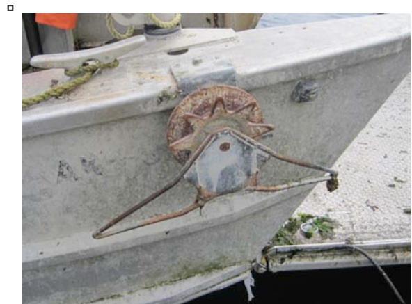
Star rollers are a great help in moving a service vessel along a longline.
