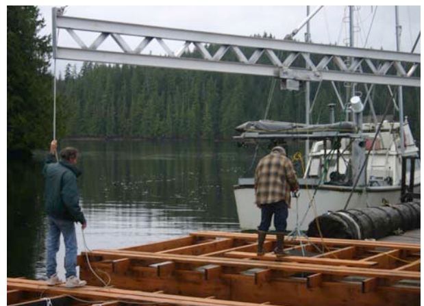
The long boom arm and hoist at Naukati make it easy to access trays from the entire raft without shifting locations. It is possible for a single operator to lift the stacks of trays and move them to the dock for tumbling and sorting.
