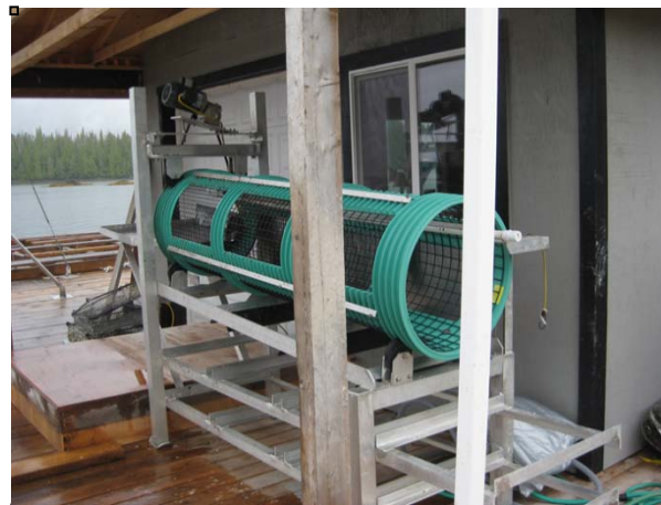
Tumbler/sorter on Mike and Kathy Sheet's farm in Sea Otter Sound in southeast Alaska. (Photo by Mike Sheets)
