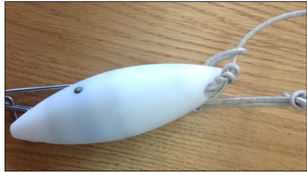
F3 pinger (about 5 inches long) used to deter marine mammals.
