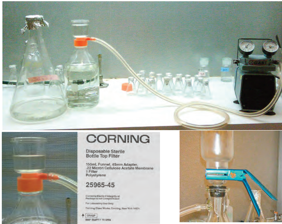
Figure 2.3. Vacuum pump assembly for filter sterilization ( 0.2 \mu\text{m} ) of nutrient media (top). Filter assemblies can be disposable (left, bottom) or reusable (right, bottom).
