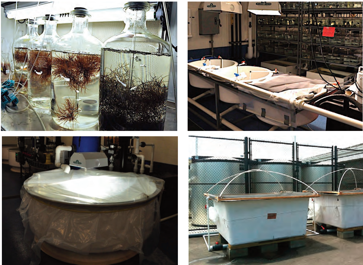
Figure 4.9. Building biomass for Gracilaria culture: Laboratory scale, small tanks, medium tanks, large outdoor seawater tanks.
