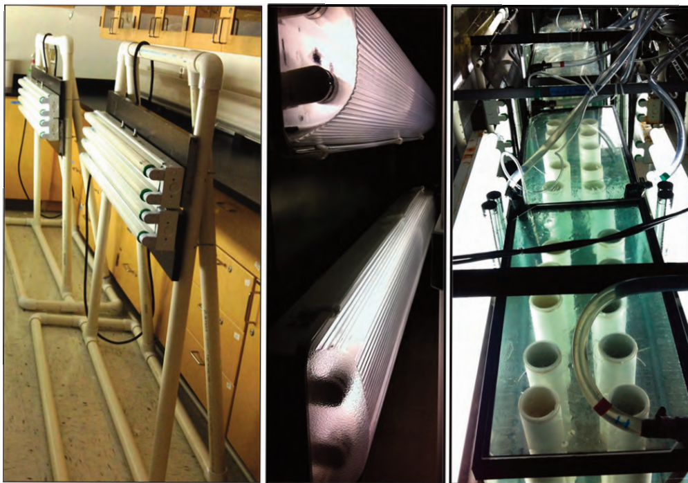
Figure 3.6. Lateral or side lighting for kelp culture systems.
