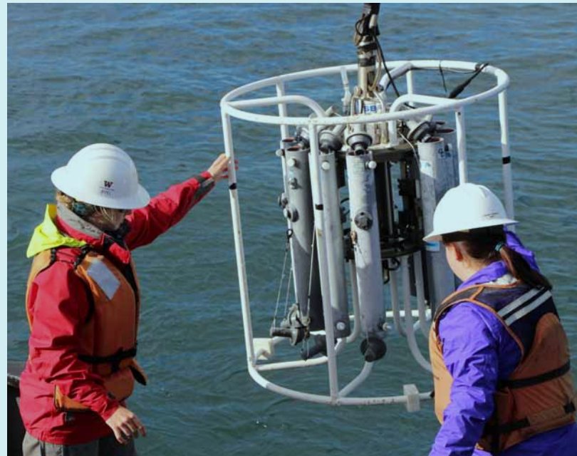
Students deploy a CTD aboard the R/V Centennial. Photo: Breck Tyler
