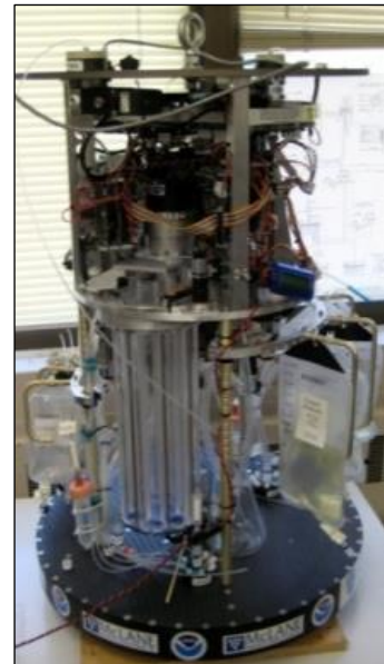
Figure 5. ESP unit without oceanographic deployment shroud at the NOAA NWFSC laboratory in Seattle.
