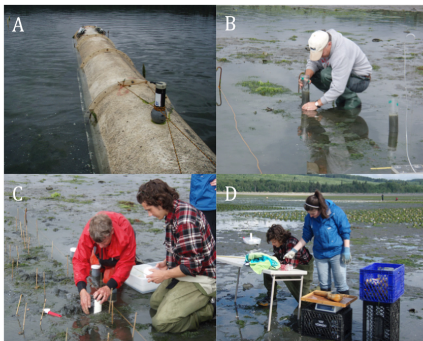
Figure 6. BEST experimental set-up and sampling activities. Panel A: tunnel at low tide; Panels B and C: collecting cores for sediment-water exchange and benthic infauna; Panel D: measuring sizes of harvested geoducks.
