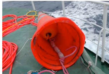
Figure 15. Modified road cone with 1.7 kg weight as a tori line towed device.
