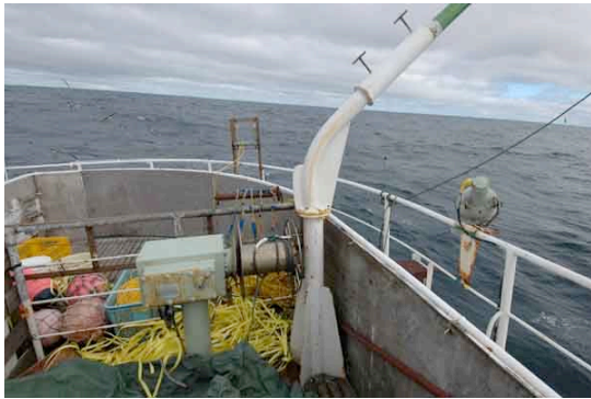
Figure 6. Port tori pole davit and winch.
