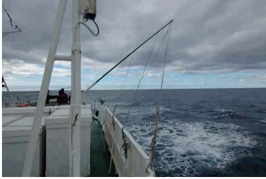
Figure 7. Port tori pole
