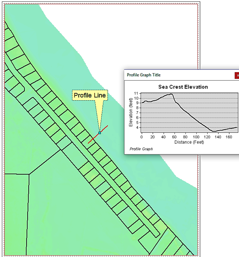
Figure 3. Example approach for estimating the sea-crest elevation for each parcel using the “profile tool” in the ArcGIS 3-D Analyst toolbox. A profile line was drawn for each parcel, and elevations along that profile extracted from a LiDAR derived digital elevation model. The peak elevation of the most seaward berm was extracted manually from the profile graph.
