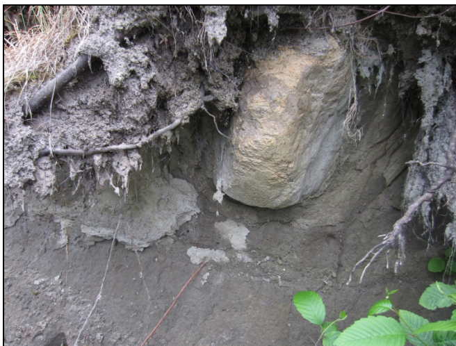
Figure 6. Exposure of till near top of bluff at assessment site. Note large boulder and spalling of fine-grained silt and clay matrix due to repeated wetting/drying of the bluff face.
