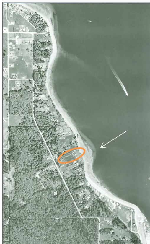
Figure 11. This 1978 Aerial view of a portion of the drift cell within which the assessed site is located shows that although the prevailing long-shore drift is northward, sediment moves southward when waves are generated by north winds. Orange circle indicates assessment property; white arrows indicate southward sediment transport.
