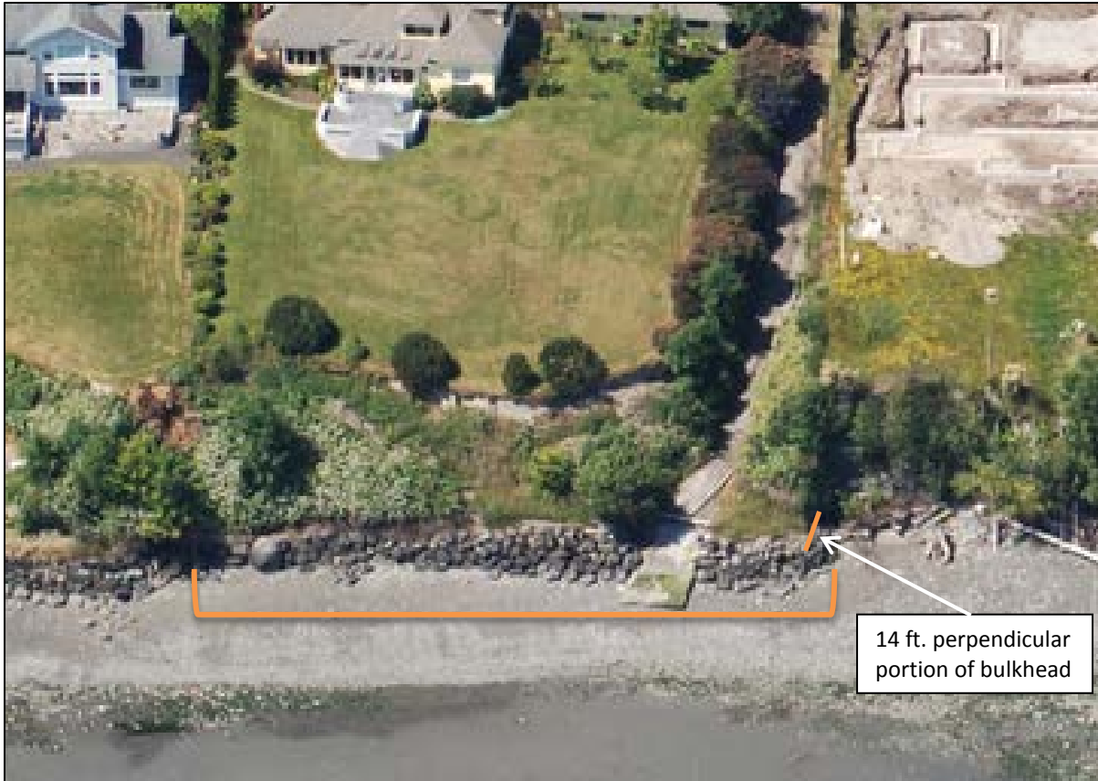
Figure 12. Dept. of Ecology oblique shoreline photo showing bulkhead, degaussing station beach access roadway, and concrete boat ramp being considered for removal and restoration – all delineated within orange line.
