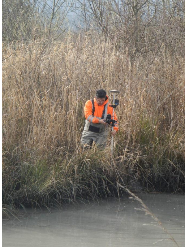
Figure 2. A ProMark 3 rover attached to a 6 foot rover pole being used by Daniel Bennett, LEKT, to survey the edge of the estuary complex.
