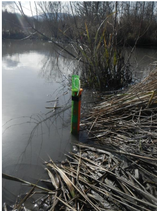
Figure 4. The staff gauge used to measure water level in the estuary complex on 8 February 2013.
