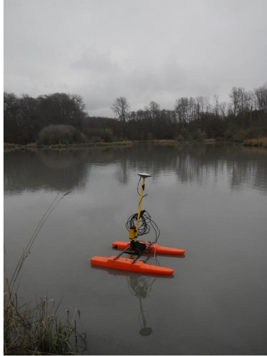
Figure 3. The Sonarmite shallow water survey system and ProMark 200 RTK-DGPS system mounted to a cata-raft.
