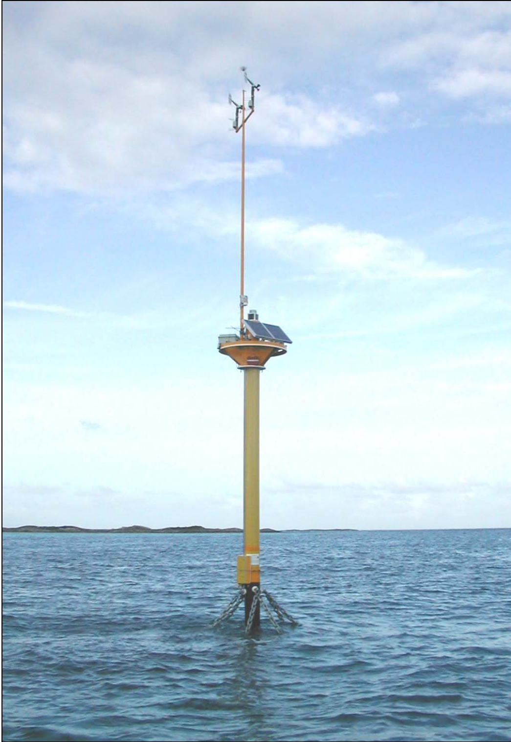
Coral Reef Early Warning System (CREWS) station near Lee Stocking Island, Bahamas.
