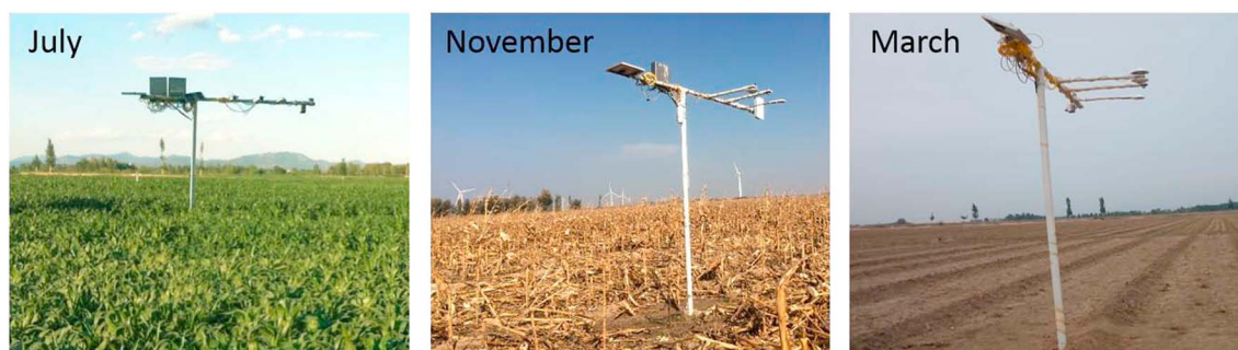
Figure 2. Photographs of WSN sites (node 5 for example) in different periods. (left to right) These pictures indicate the surface conditions during vegetation period, mixed surface period, and bare soil period, respectively.
