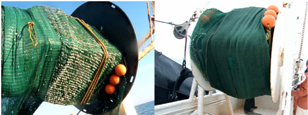
Figure 8. The FFF-TED stored on an 8 ft (3.6 m) wide reel (left) and narrower 4.5 ft (2 m) wide reel (right).
