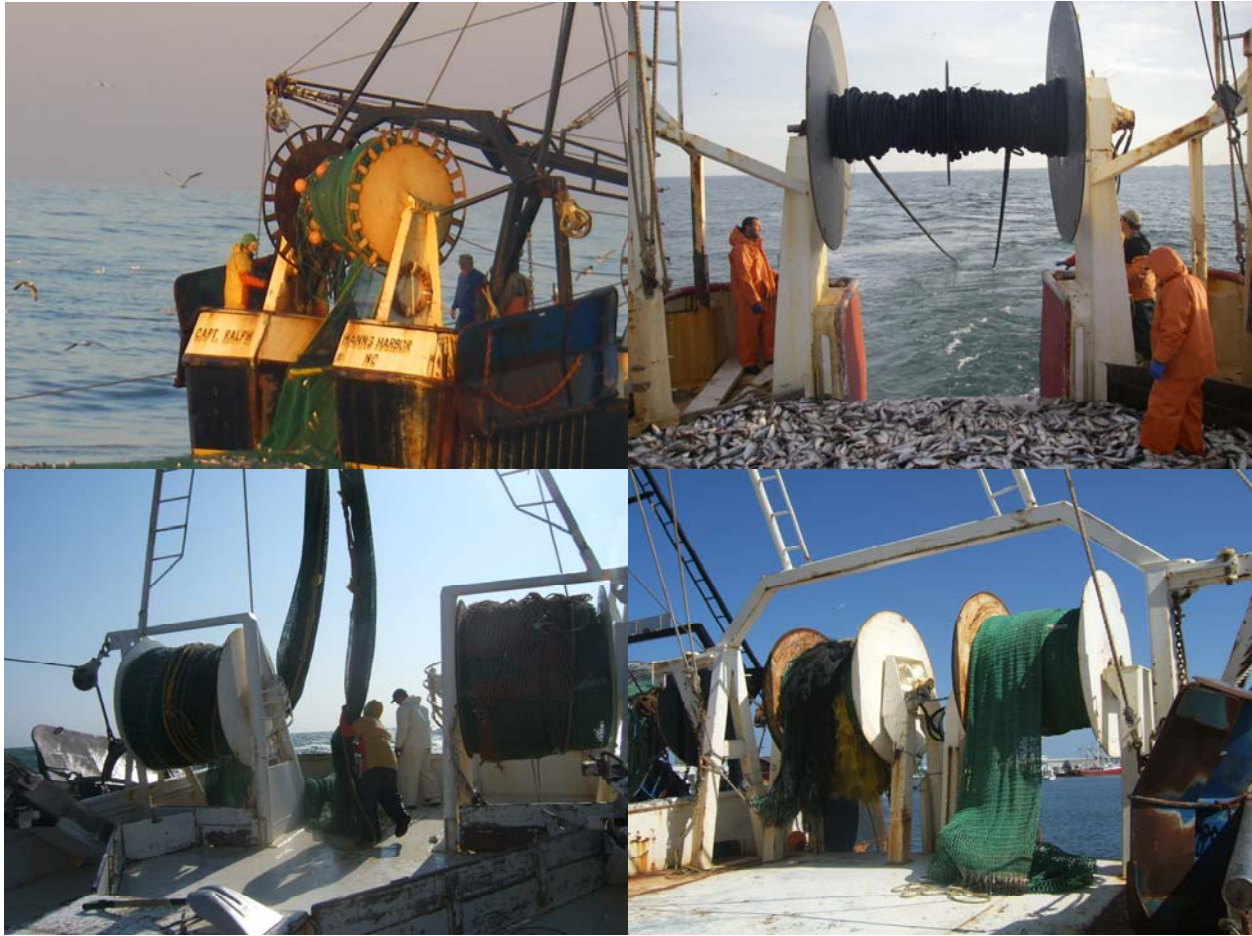
Figure 7. Net reel configurations of the four vessels contracted to conduct TED usability testing.
