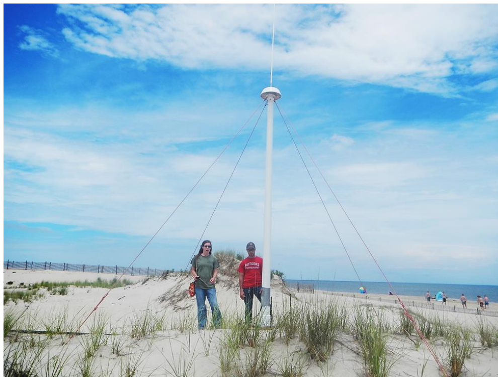
Figure 3-1. A SeaSonde 25 MHz combined transmitting and receiving antenna deployed at Cape Henlopen, Delaware.
