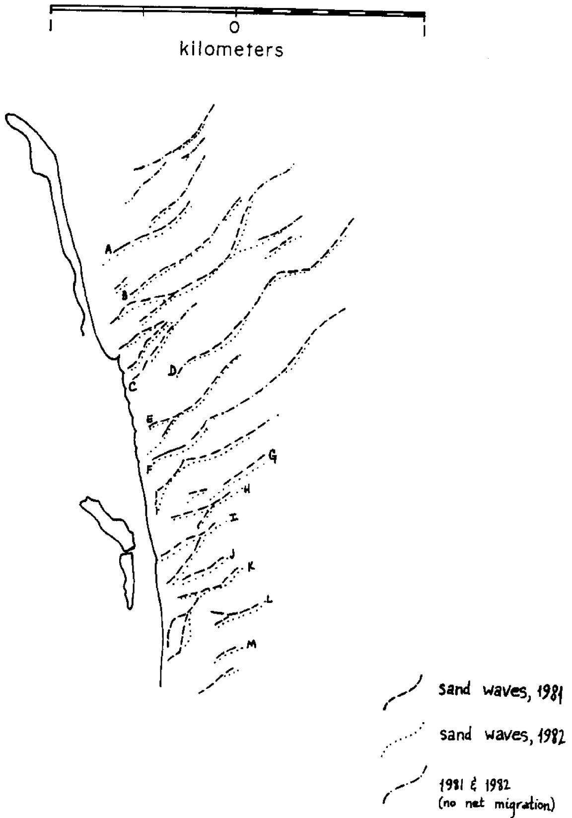
Figure 18. Sand wave migration patterns in the Popponeset study area for the period 1981-1982. Sand wave labels are as referred to in table 3.
