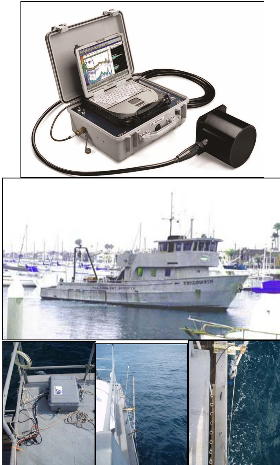
Figure 7. BioSonics DT-X unit with hydrophone (top), RV Yellowfin (middle), and BioSonics transducer unit mounted to by retractable boom to the port side a midship of vessel (bottom).
