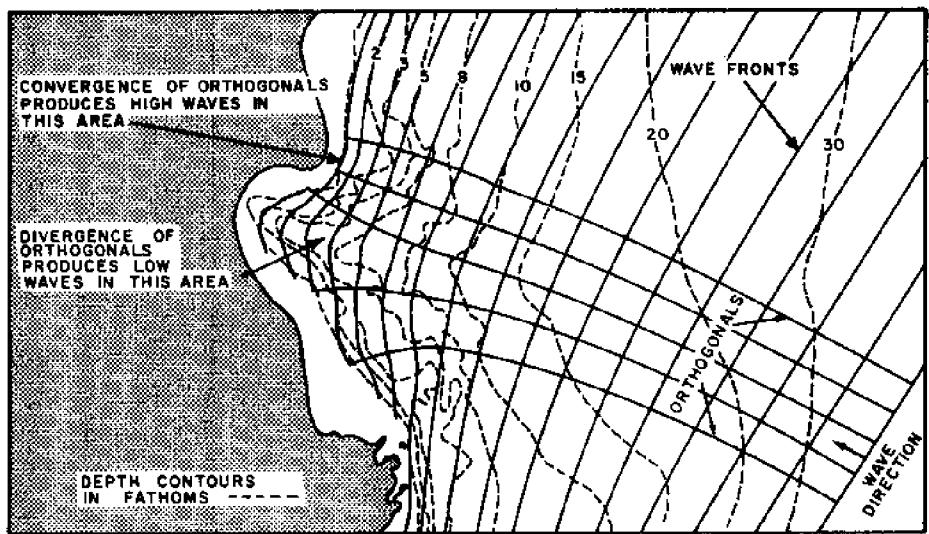
**Figure 2.** Correlation between measured wave heights and computed wave heights (as determined from manually-drawn refraction diagrams) for specific wave conditions. Note that low wave heights occurred in areas of wave ray divergence and larger wave heights in areas of wave ray convergence (modified from Munk and Traylor, 1947, Fig. 16).
