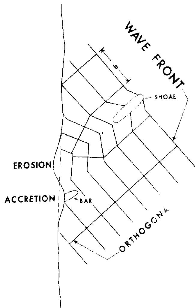
Figure 8. Continental shelf contour diagrams summarizing computations of wave parameters made in the VSWCM along wave rays (Goldsmith, et al., 1975).
