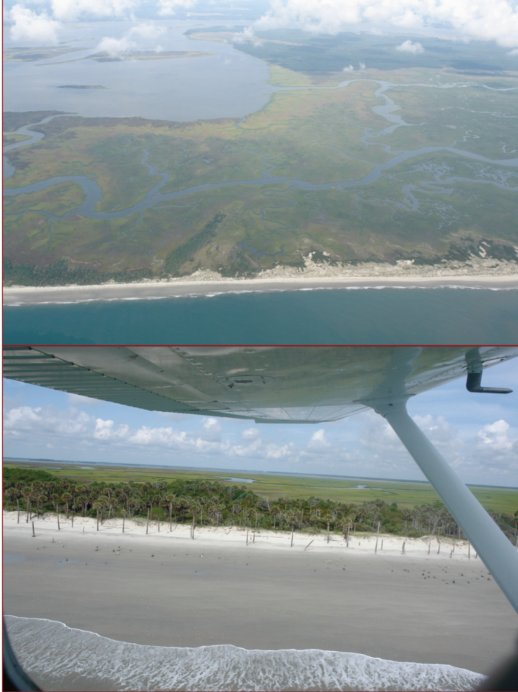
Figure 11. The central section of North Island consists of a narrow beach with a small dune system immediately adjacent to salt marsh vegetation (top). Historical shorelines (see Figure 9), remnants of trees in the intertidal zone, presence of trees on the berm, and erosion of the primary dune indicate this section of North Island is net erosional. Photographs: Aug 2009.
