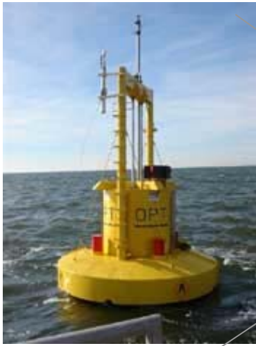
Figure 5 PowerBuoy Device Proposed for the Ocean Power Technologies Wave Park -Reedsport, Oregon (Reedsport OPT Wave Park, LLC 2010).
