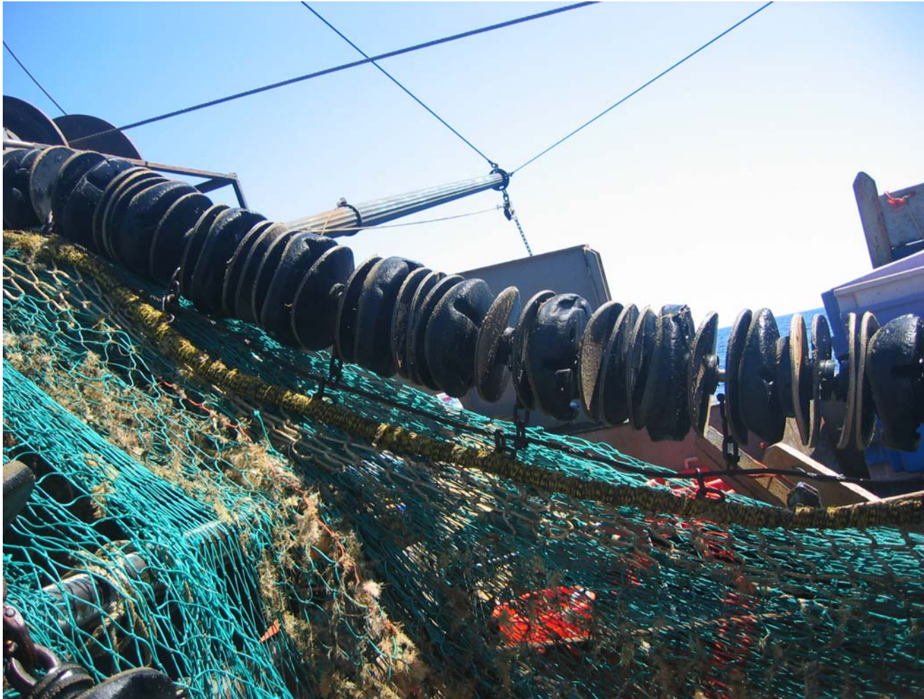
Figure 6. Photo of the rockhopper sweep of the control net showing the five 16 inch rubber discs per bight in the center.
