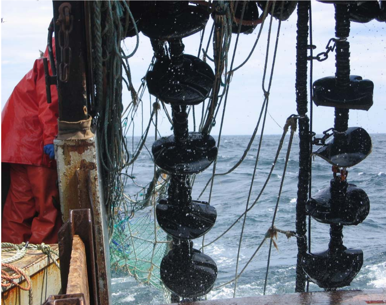
Figure 9. Photo of the rockhopper sweep of the experimental net, the “Eliminator Trawl,” showing the one 16 inch disc per bight in the center.
