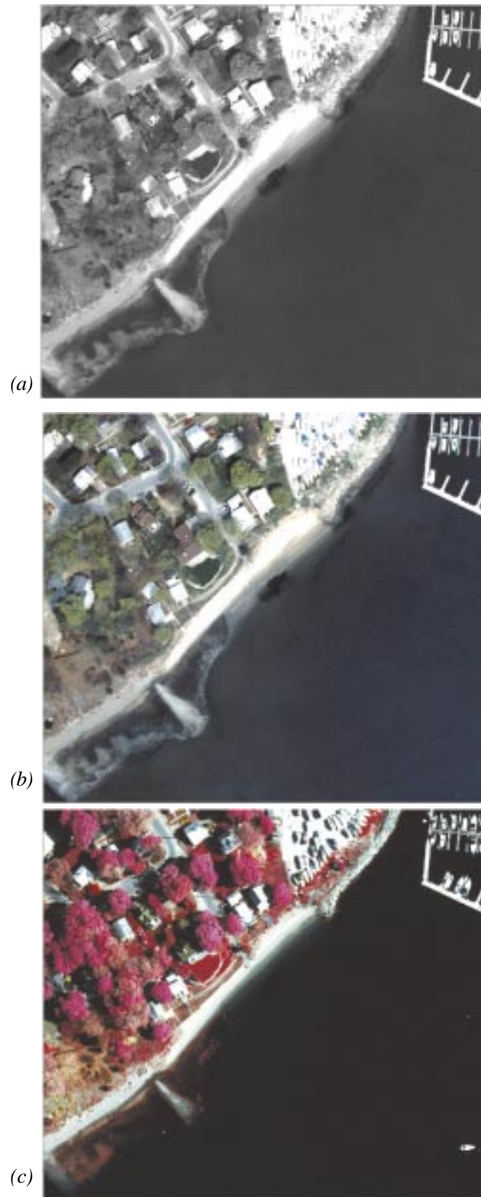
Figure 2. Representative images from the (a) panchromatic, (b) natural color, and (c) color infrared orthophotography.
