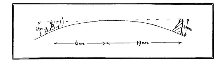
Note that irregular atmospheric conditions and the reflecting characteristics of the target can greatly affect the range. For instance, the echo strength from an iceberg is often only about 1/50 that received from a steel ship of similar size.
