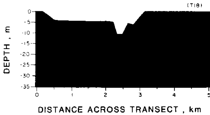
Figure 15. Cross-sections across the Providence River and Mount Hope Bay. Transects 1,2,17,18 (see Figure 10). Vertical exaggeration 175X for transects 1 and 2, 60X for 17 and 18.
