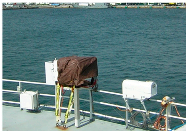
FIG. 3. (left) Unenhanced photograph of the forward of the NOAA research vessel Ronald H. Brown , taken during AEROSE-III, on the afternoon of 13 May 2007, when there is a strong Saharan dust aerosol outflow pulse (Nalli et al. 2011). (right) The M-AERI is mounted on the starboard side railing of the O2 deck of the ship.
