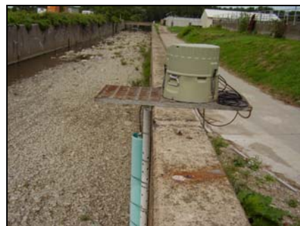
Figure 8. ISCO 6712 sampler used to collect storm water from Mill Creek
