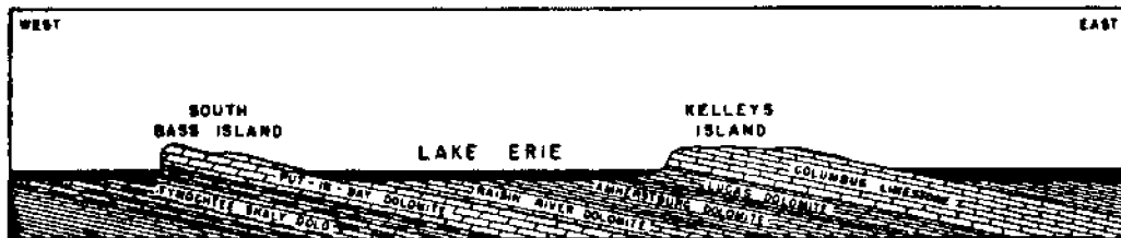
Figure 24. Geologic cross section of the bedrock underlying South Bass and Kelleys Islands (Carman 1946). The structure of the bedrock has resulted in the cuesta shape of the islands with cliffs on the west sides and gentle slopes on the east sides.
