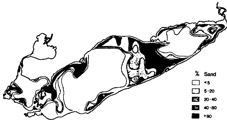
Figure 3a. Distribution of Percent Sand-size Fraction in the Surficial Sediment of Lake Erie.
