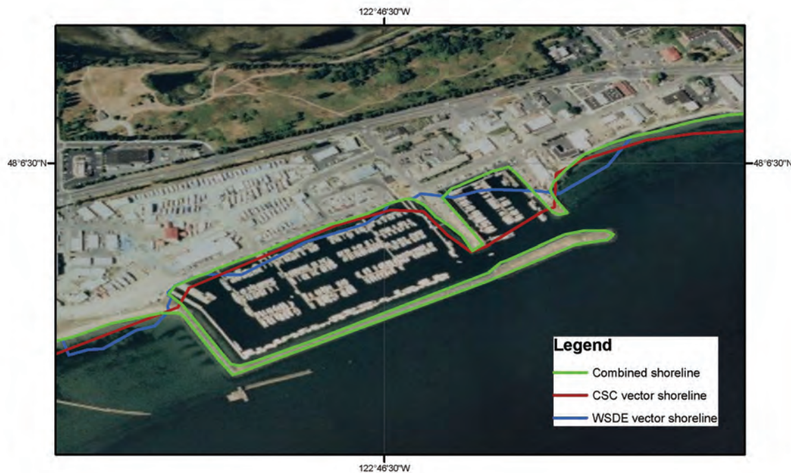
Figure 5. Combined shoreline of Port Townsend Harbor (green line) shown with ESRI World 2D Imagery. Piers are not included in the shoreline as water can flow beneath them, but large rocks and breakwaters were included as they are solid structures.
