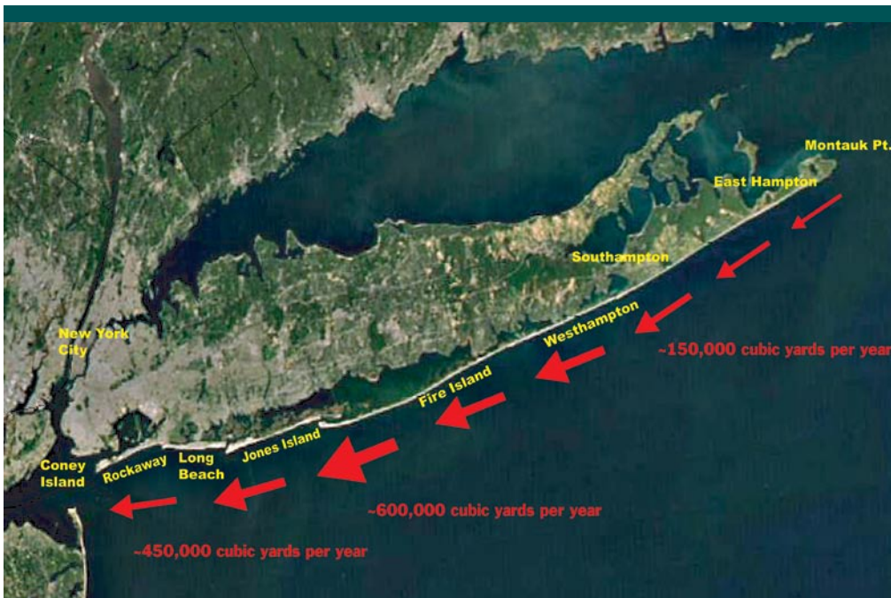
Figure 18. Sand moves in both directions along the shore, but generally more sand moves to the west than to the east resulting in a net westerly transport. There is considerable uncertainty in the values shown here due to variability in the rates of movement at different times and places and difficulties associated with trying to measure the amount of sand moving along the coast.
