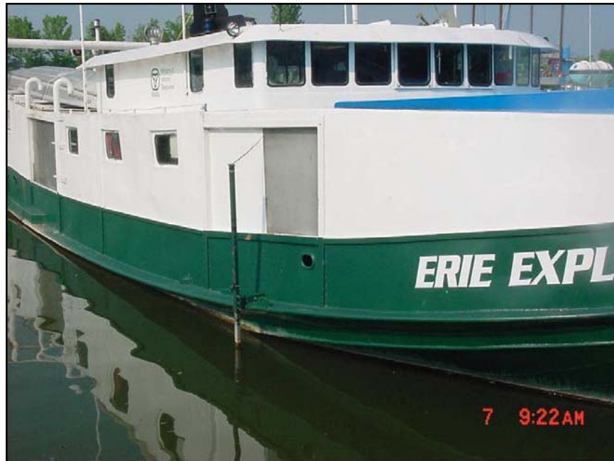
Fig. 7. Example of a pole-mounted transducer deployment.
