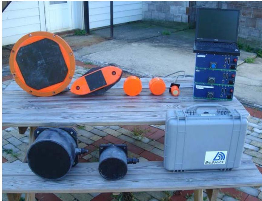
Fig. 2. Example of transducers made for different frequency output. Note that lower-frequency transducers are larger in physical size. Top row (L to R): Simrad 38 kHz, 70 kHz, 120 kHz, 200 kHz, and 710 kHz, all approximately 7° beam width (70 kHz at 11°). Bottom row (L to R): BioSonics 120 kHz (7° beam width) and 430 kHz (6° beam width). Photo by Tom Brooking, Cornell University Biological Field Station, Bridgeport, NY, 13030.
