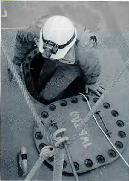
A researcher enters a ship's ballast tank to collect sediment samples for analysis of living organisms.
