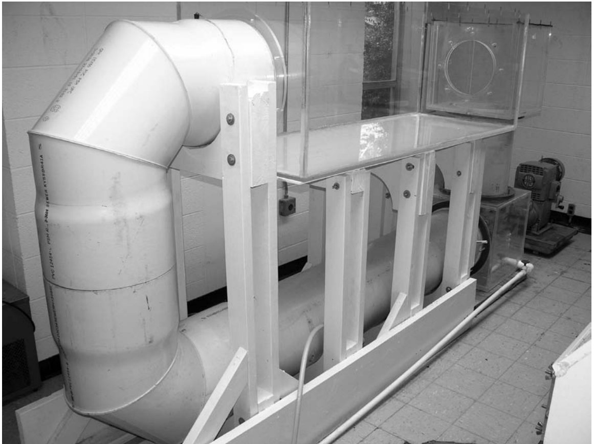
Figure 1. The Brett swim tunnel used for red snapper critical swimming speed determinations.
