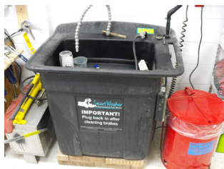
Bioremediating parts washer at Washburn Marina. Photo Credit: Gene Clark, UW Sea Grant Institute.
