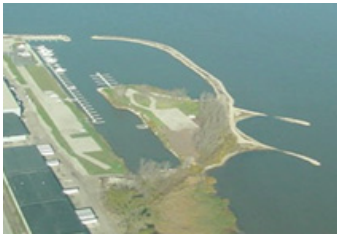
Rock groins extending from South Bay Marina create a captive beach for wildlife use. Photo credit: Dave Wentland.
