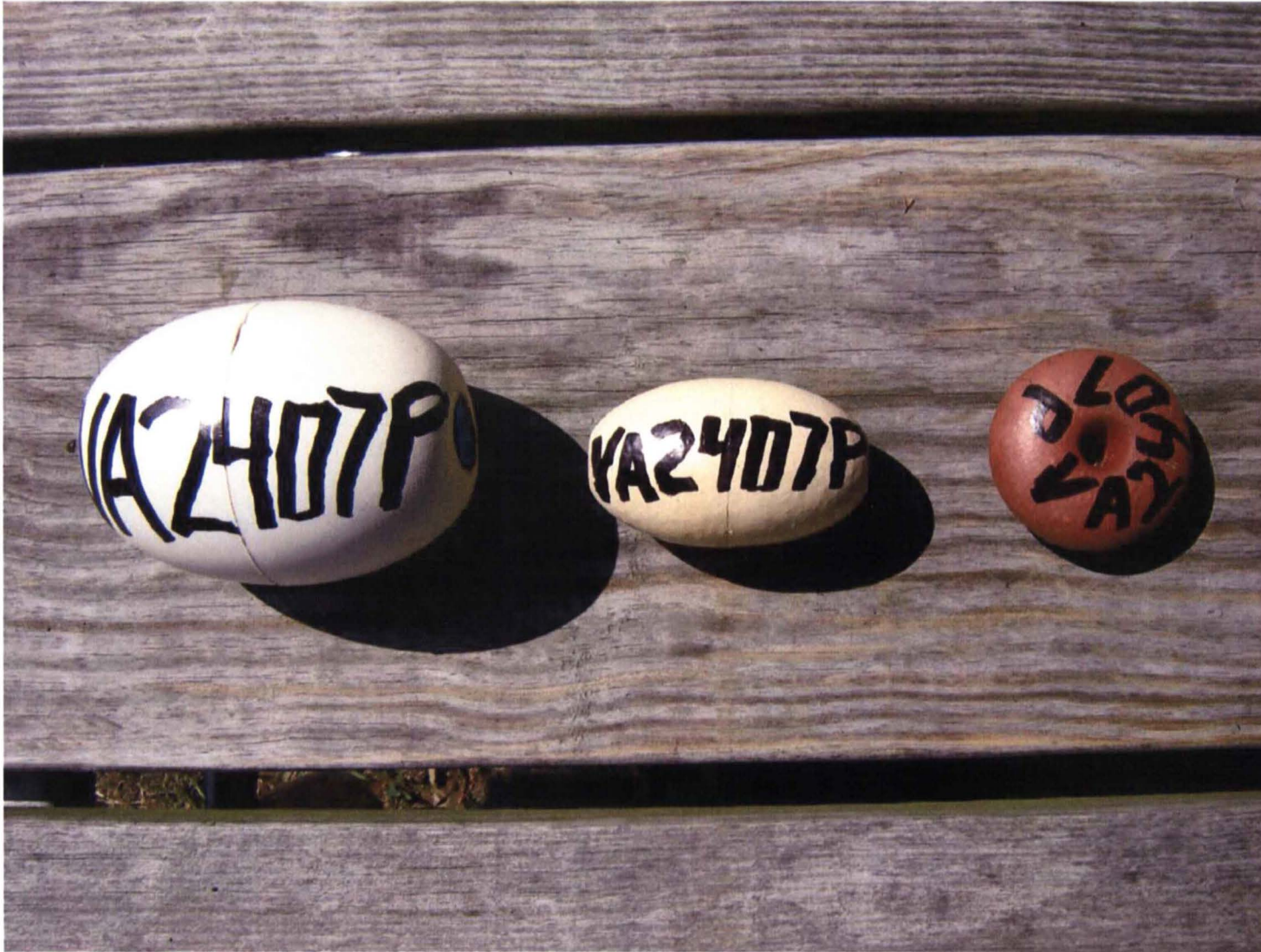
Figure 1. Float marked with Sharpie® permanent marker are shown. Float on left is type used on float nets, middle is hard float placed on sink nets, and right is donut or skiff float. This type is relatively soft and deforms under pressures of net reels.
