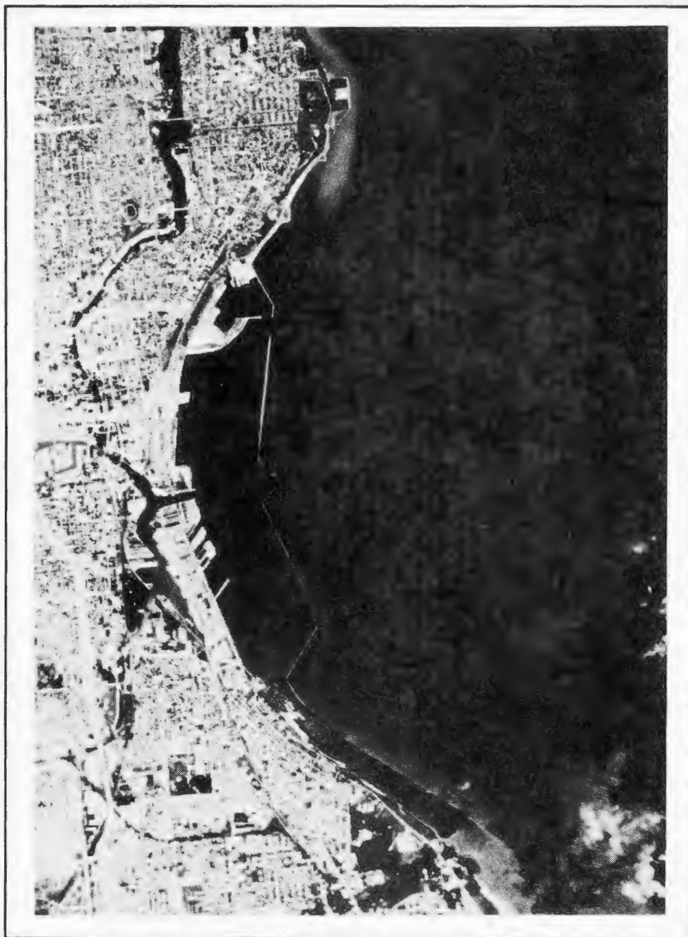
Figure 6. Milwaukee Harbor and Lake Michigan: enlarged portion of a 9-inch square transparency (color infrared, plus green band) taken from a height of 60,000 feet on Sept. 22, 1972, after 3.81 inches of rainfall during the preceding 6 days. A turbid plume is leaving the harbor and travelling southward. (Copy of NASA photograph in Engineering Library, UW-Madison.)
