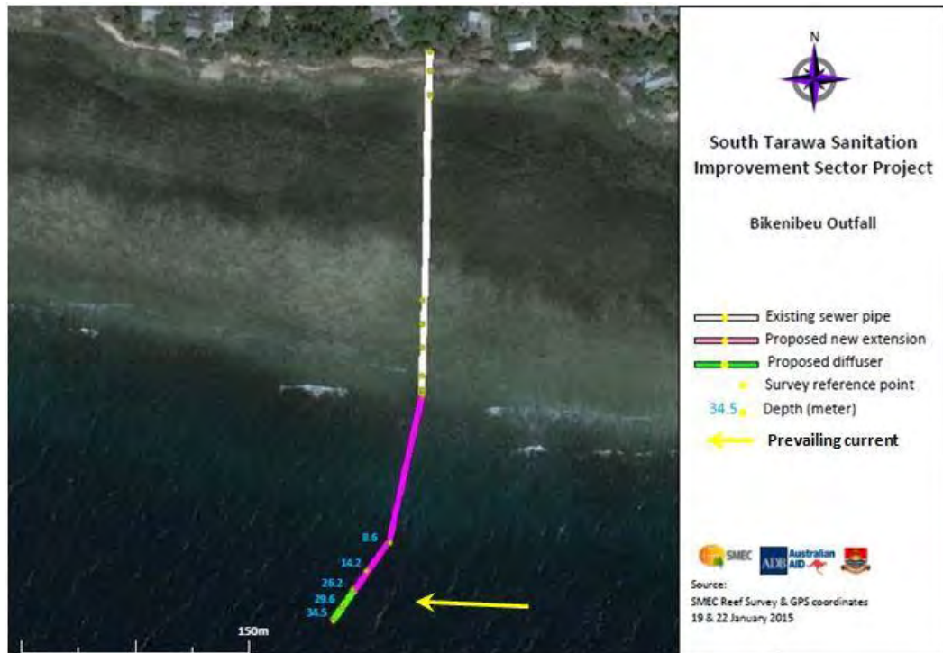
Fig. 4.3.2 Existing Outfall Pipe and Proposed Extension at Bikenibeu (note: reference depths not corrected for 0 datum)
