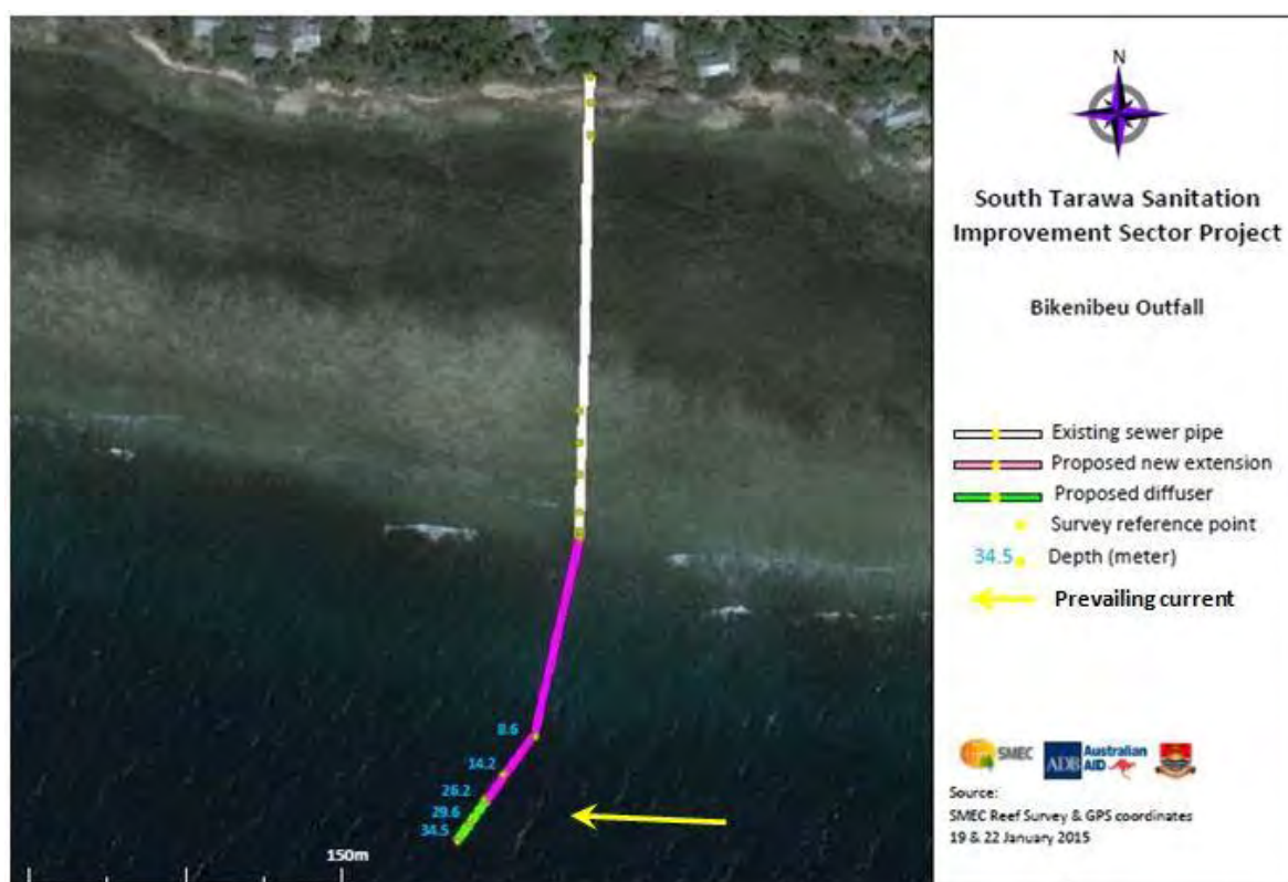
Fig. 4.3.33 Existing Outfall Pipe and Proposed Extension at Bikenibeu (note: reference depths not corrected for 0 datum)
