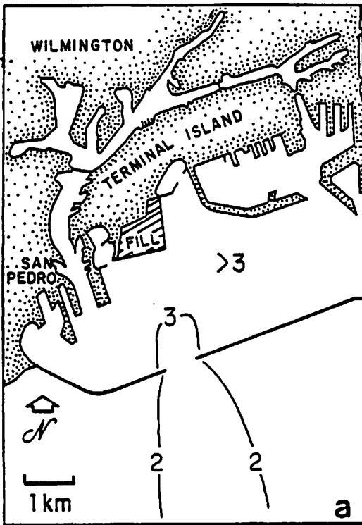
FIGURE 15. SIMULATIONS PREDICTED THAT DIRECT CANNERY DISCHARGE OF 10 MGD EFFLUENT (b) WOULD BE EXPECTED TO RESULT IN HIGHER LEVELS OF AMMONIUM ( \mu\text{g-at } N \text{ l}^{-1} ) RELATIVE TO BASELINE TITP DISCHARGE WITH NO CANNERY EFFLUENT (a).
