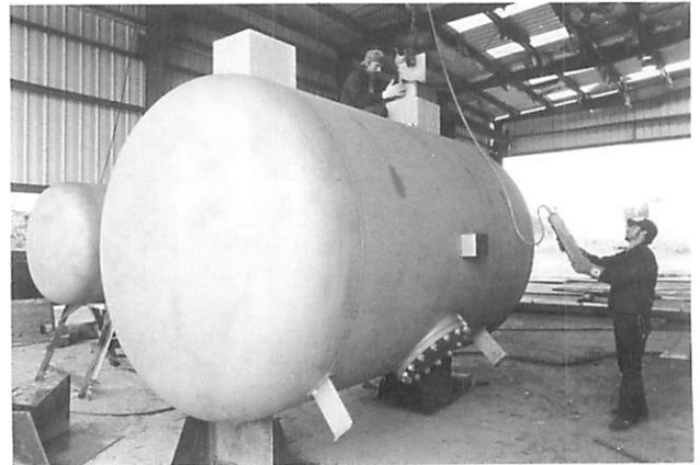
Left: Sea Grant researcher C. Everett Brett of the University of Alabama examines the heads of specially designed cryogenic tanks for storing super cold LNG (liquefied natural gas) on board a new breed of shrimp boat that could cut 45 percent off Gulf of Mexico shrimpers' annual operating costs. Right: Workers prepare for pouring high density foam mounts for the completed tanks. Below: The larger of the two tanks is installed in the vessel's forepeak.
