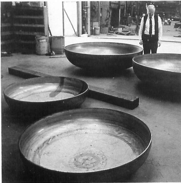
Left: Sea Grant researcher C. Everett Brett of the University of Alabama examines the heads of specially designed cryogenic tanks for storing super cold LNG (liquefied natural gas) on board a new breed of shrimp boat that could cut 45 percent off Gulf of Mexico shrimpers' annual operating costs. Right: Workers prepare for pouring high density foam mounts for the completed tanks. Below: The larger of the two tanks is installed in the vessel's forepeak.
