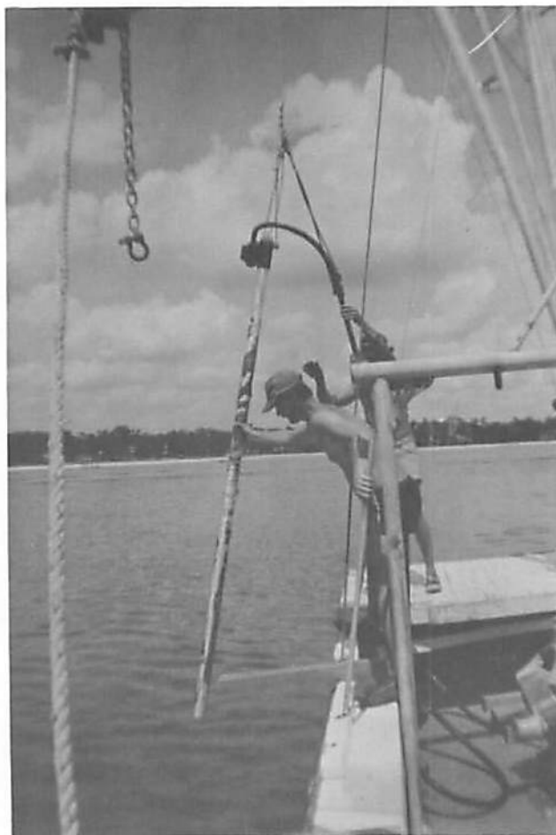
Collecting a vibracore in Mississippi Sound.
