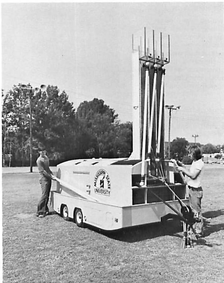
A strange contraption, this field unit was constructed to investigate electrolysis as a method of economically treating seafood processing waste water.
