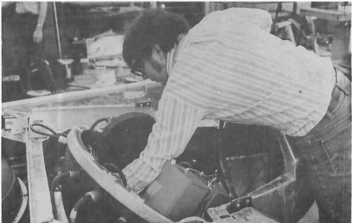
Figure 7. Technician making an adjustment on the intervolemeter which controls the time between consecutive data pictures.
